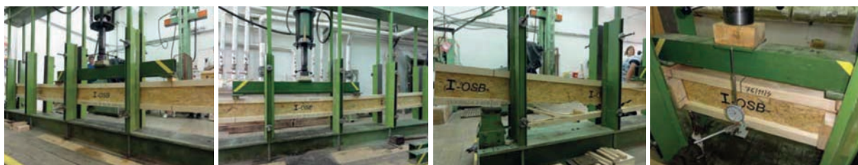
Testing and certification of the I-OSB™ wooden beams
